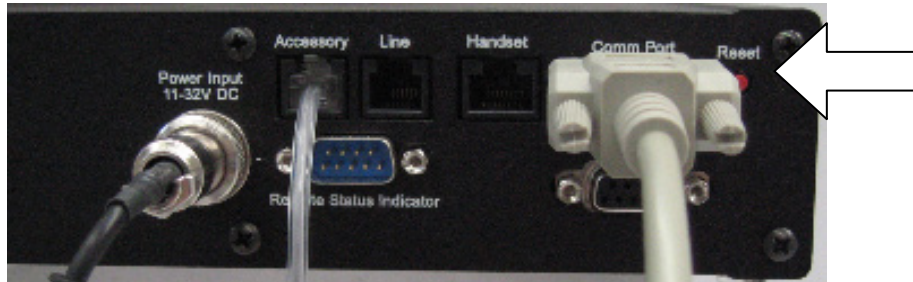
Figure: Serial cable connected to Comm Port
